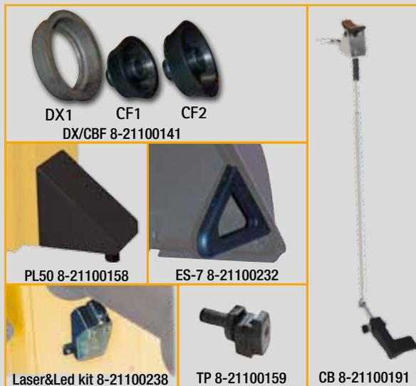
EN → •DX/CBF Centring accessory for van and off-road wheels with central hole with  $\varnothing 117 \div 173$  mm •PL50 Base for balancing wheels up to 50 kg without fastening the machine to the ground •ES-7 AWD automatic sensor •Laser&Led kit Inside wheel LED light and LASER pointer kit •TP STD ALU weight-holder terminal •CB Pedal wheel holder shaft locking brake.
